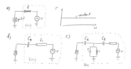
If the impedance of the environment is purely resistive, e.g.  $Z(\omega) = 50 \Omega$ , the decay rate  $\Gamma = 1/T_1$  is frequency independent (see Figure a).
