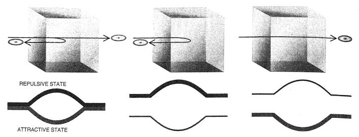
EMPTY CAVITY can repel or attract slow-moving, excited atoms. The strength of the coupling between an atom and a tuned cavity typically vanishes at the walls and reaches a maximum in the center. (Curves at the bottom show the energy of the atom-cavity system as a function of the atom's position within the cavity.) The change in energy results in a force
