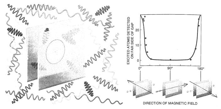
EXCITED ATOM between two mirrors (*left*) cannot emit a photon. The atom is sensitive to long-wavelength vacuum fluctuations whose polarization is parallel to the mirrors, but the narrow cavity prevents such fluctuations. Atoms passing through a micron-wide gap between mirrors have remained in the ex-
