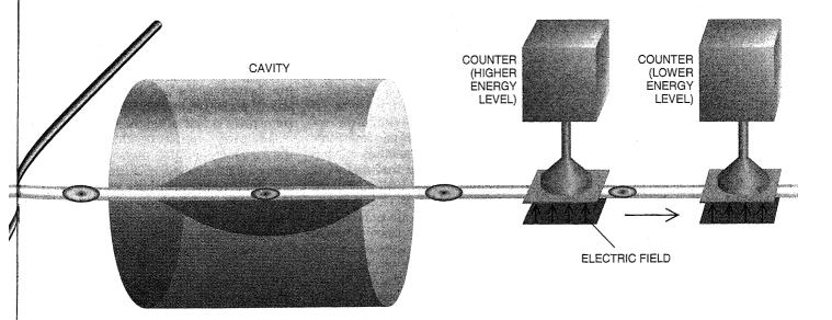
MICROMASER uses an atomic beam and a superconducting cavity to produce coherent microwave radiation. A laser beam (*left*) strikes atoms coming out of an oven and excites them into high-energy Rydberg states. The atoms pass one at a time through a cavity tuned to the frequency of a transition
