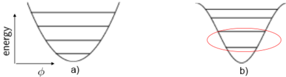
FIGURE 2.3.1. a)Harmonic energy spectrum b)An-harmonic energy spectrum
