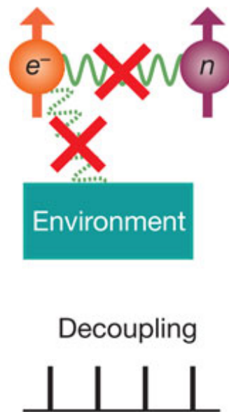
b Protected storage: Decoupling
