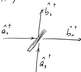
$$\begin{aligned} \hat{a}_1^+ &\xrightarrow{\text{BS}} \frac{1}{\sqrt{2}} (b_1^+ + b_2^+) \\ \hat{a}_2^+ &\xrightarrow{\text{BS}} \frac{1}{\sqrt{2}} (-b_1^+ + b_2^+) \end{aligned}$$
