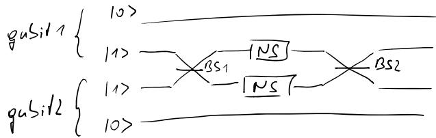
non-linear sign gate (NS)  $\alpha|0\rangle + \beta|1\rangle + \gamma|2\rangle \rightarrow \alpha|0\rangle + \beta|1\rangle - \gamma|2\rangle$
